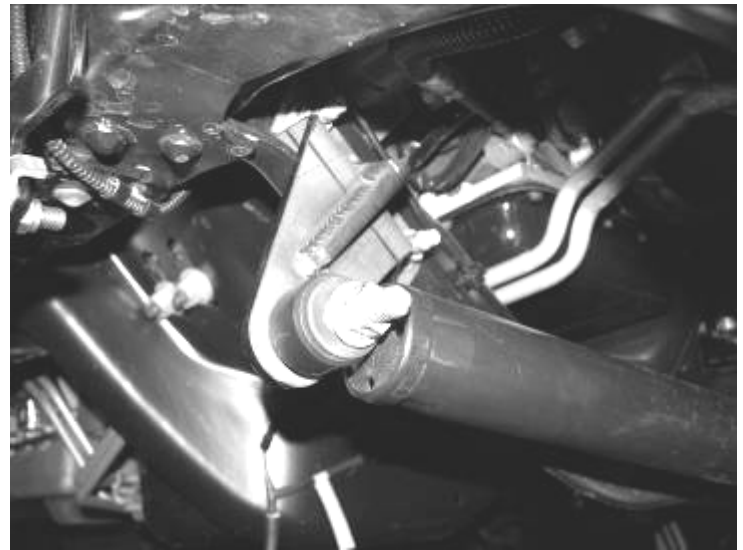
Picture Shown with Factory Stabilizer re-installed
