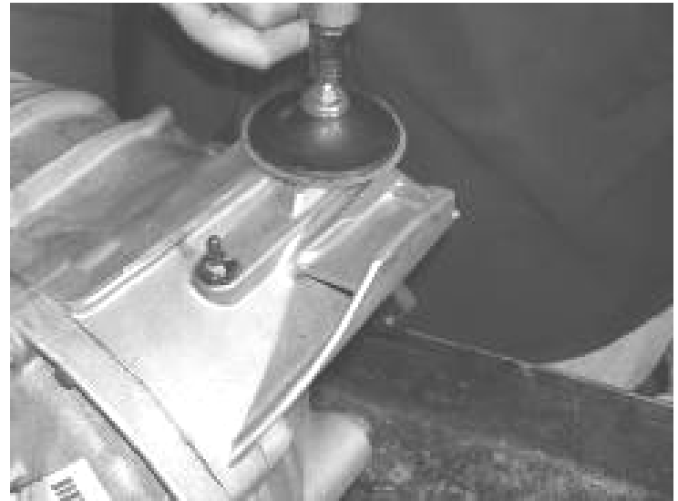
After Cut & Sanding Surface Smooth
