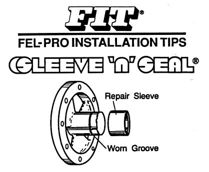
To insure proper function of this product on this application this sleeve must be aligned perfectly, straight and true and fully bottomed on the balancer hub before assembly.
