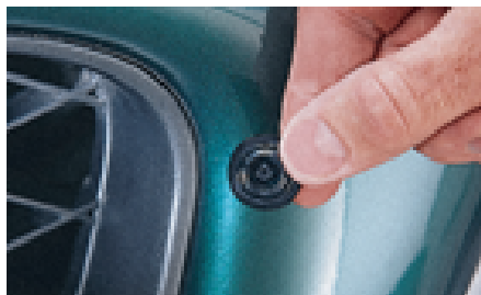
Adhere Stick-a-Stud™ fasteners to vehicle
