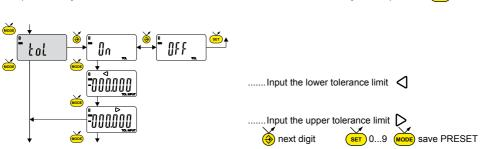
To input or modify the tolerance limits,  $t_{al} \rightarrow l_{a}$  mode should be selected, followed by a short press on (
