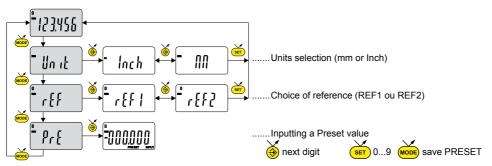
Note: It is possible to assign a different preset value to each of the 2 References. Similarly, different tolerance limits can be assigned to References 1 and 2.
