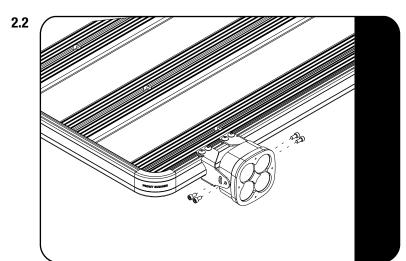
Place your Baja Light between the Mounting brackets and secure using the fasteners supplied with the light.
