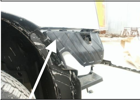
Step 1 Remove plastic shield above chrome bumper
