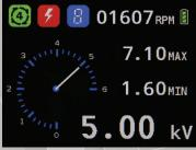
Analog gauge and digital readout with maximum and minimum.
