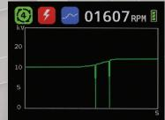
Unique chart mode makes easier to detect intermittent or infrequent failures and misfires.
