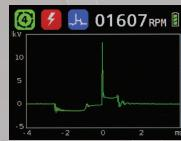
Displays secondary ignition waveforms.
