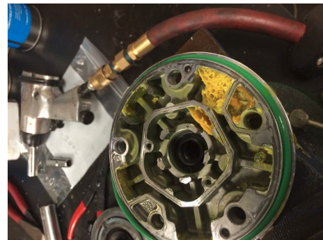
Pictured above: Solidified sealant trapped in the cylinder and cylinder head
