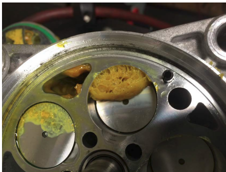
Pictured above: Solidified sealant trapped in the cylinder and cylinder head
