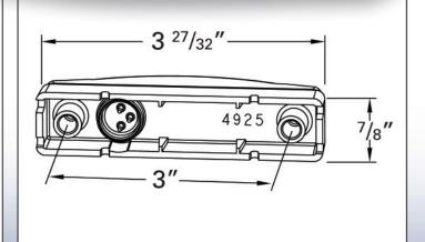
Material: Polycarbonate Finish: Red /Yellow FMVSS/SAE Code: P2, U
