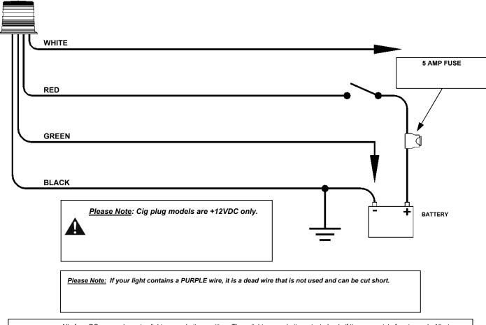
All of our DC powered warning lights are polarity sensitive. These lights are polarity protected *only if the appropriate fuse* is used. All wires connected to the positive terminal of the battery should be fused <u>at the battery</u> for their rated load. **Testing the light before this fuse is properly installed will void the warranty on the light.**
