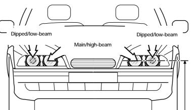
The dipped/low beam bulb must be between 22 inch - 54 inch (559 mm - 1372 mm) above the road surface
