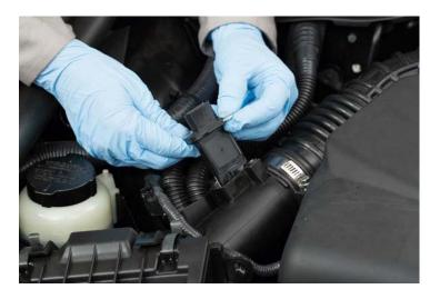
4. Slide the air flow sensor into the air cleaner case.
