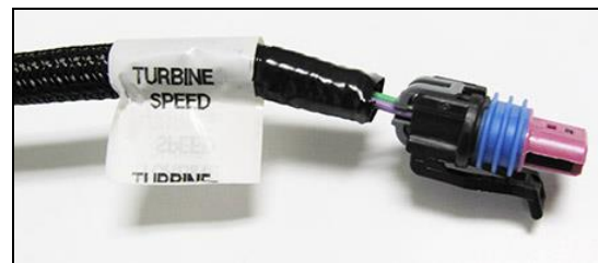
Turbine Speed Sensor
