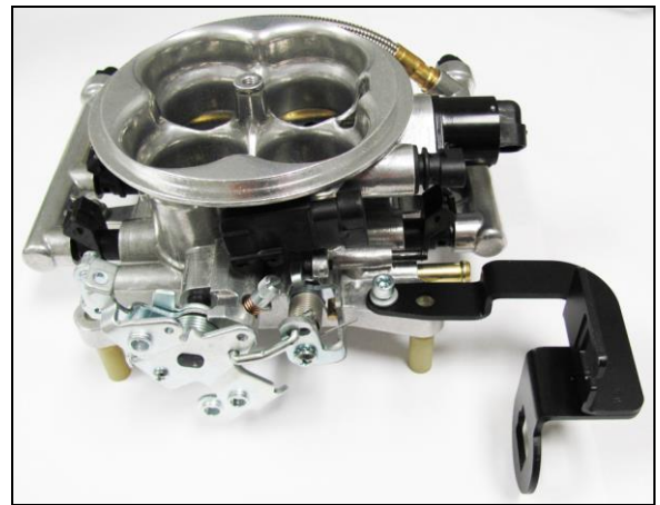
Bracket Installed (Throttle & Trans. - Item 11)
