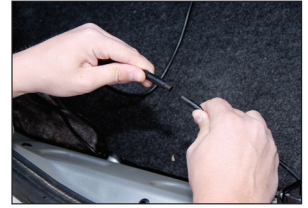
Connect wire from main bracket to the wire coming from the monitor
