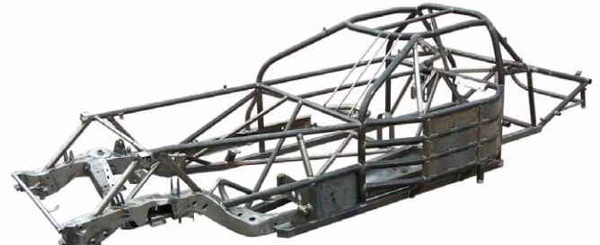
Modified Chassis with Impala Frame
