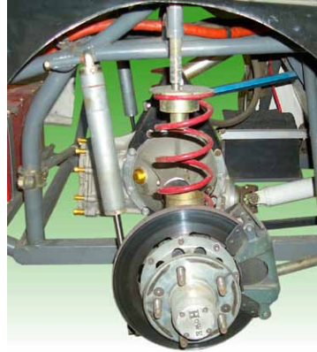
Coil Rear Suspension with Lift Bar
