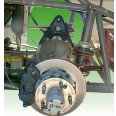
Coilover Rear Suspension with Standard 3rd Link
