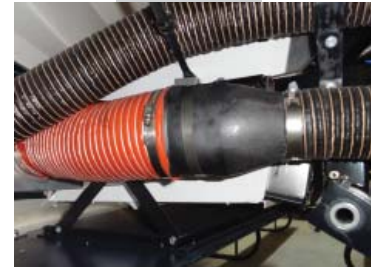
4-1/2" to 3" Brake duct adapter - no fan.
