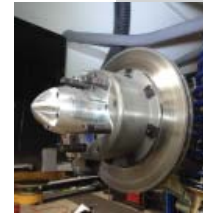
4-1/2" to 3" Brake duct adapter - no fan.
