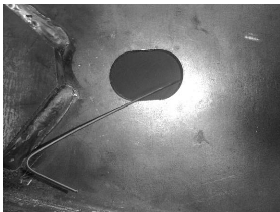
Bend end of pull wire to prevent from going through slot in bracket and hole in frame.
