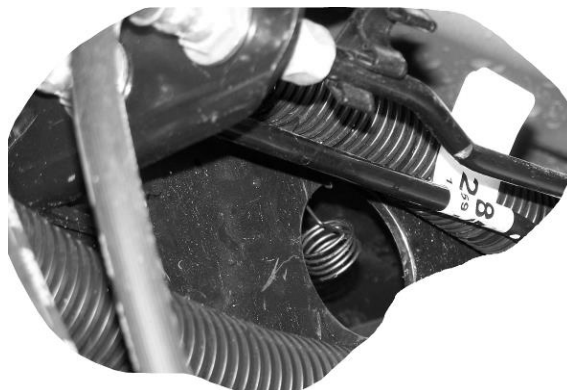
Guide pull wire coils through hole on inside of frame.
