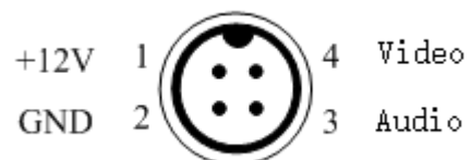
AV-OUT Monitor Interface
