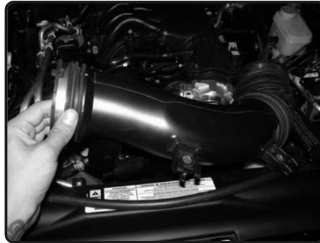
3. Remove the air duct from the throttle and air box. An intake air temp sensor will need to be removed on the next step.
