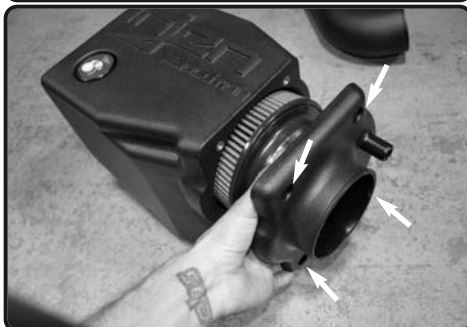
10. Insert the filter into the Injen air box. Use four M6X20 bolts and secure the Injen plenum to the Injen air box.
