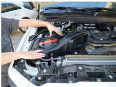
15. Line up the grommets on the air box to the factory studs then press down on the air box.
