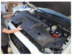
3. Using a flathead screwdriver or prying tool remove the 12 push clips holding the air scoop cover then remove air scoop cover.
