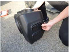
8. Press the air inlet plugs on to the Injen air box. OPTIONAL: Remove the air inlet plugs for more air flow and sound.
