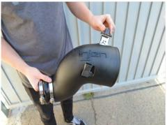
11. Install the factory MAF and IAT sensor on to the Injen tube . Then secure both senors using the provided M4 button head screws.
