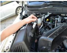
5. Remove the screws holding the MAF and 6. Remove the factory air box. IAT sensor then remove both sensors. Both sensors will be reused on the Injen tube.
