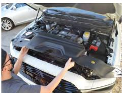
19. Reinstall the air coop cover and secure using the 12 factory push clips.
