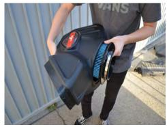
13. Install the twist lock filter on to the Injen air 14. Press the Injen tube on to the twist box. Once seated, rotate the filter a 1/4 turn in either direction so the filter can lock into place.
