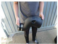
10. Press the 4.0" Hump hose on to the Injen tube then secure it using the provide clamps.
