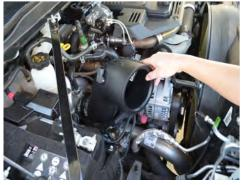
12. Attach the Injen tube to the turbo. Do not fully tighten clamps until the air box is installed.
