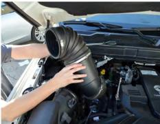
2. Loosen the two clamps holding the stock tube to the air box and turbo inlet. Then remove the tube.
