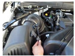
1. Disconnect the MAF harness and the Temp sensor harness
