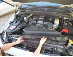
18. Install the factory scoop and secure using the factory bolts.
