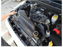
4. Remove the two bolts holding the factor air scoop then remove the factory air scoop.
