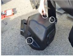
9. Install the three factory grommets onto the Injen air box.
