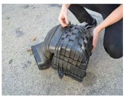
7. Remove the three grommets from the factory air box. They will be reused on the Injen air box.
