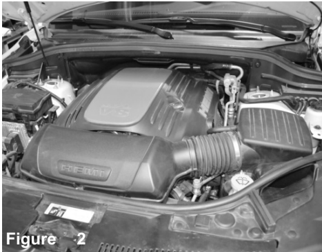
Figure 3 Lift up and remove the engine cover.
