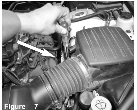
Figure 7 Loosen the clamp on the air box.
