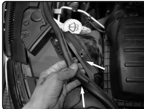
7. Carefully pull back the rubber hood line trim from the air box ram inlet.
