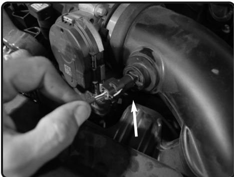
5. Disconnect the temperature sensor harness
