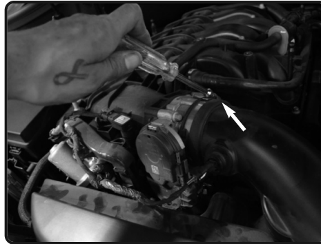
3. Loosen the clamp on the throttle body.
