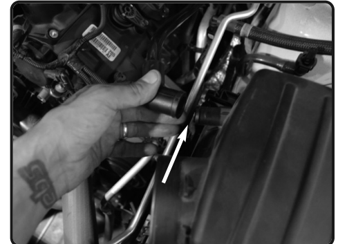
8. Pull back the crank case line from the air box.
