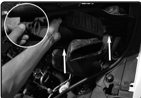
9. Lift up and remove the air box out of the vehicle. Remove 1 of the grommets on the bottom of airbox that will be used on the new heatshield.
