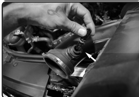
10. Turn and remove the temperature sensor out of the intake tube.
