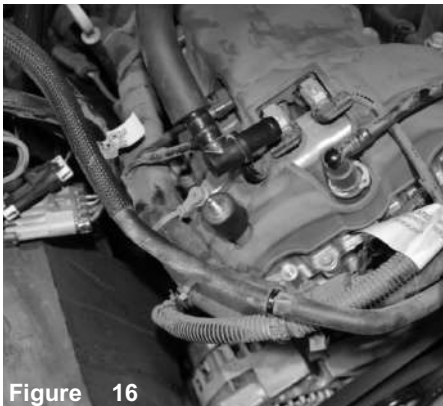
Figure 16 Secure and tighten the vibramount.
