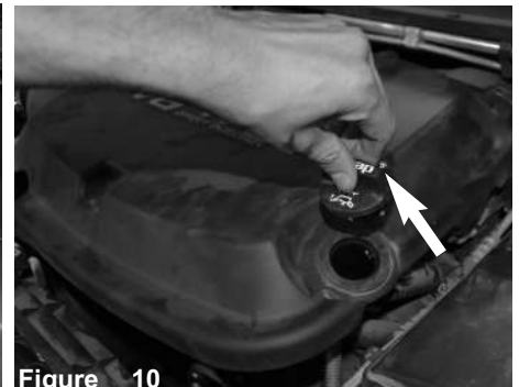
Figure 10 Remove the oil cap.
