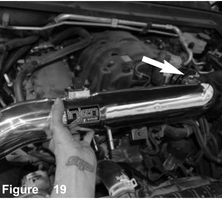
Figure 16 Secure and tighten the vibramount.
