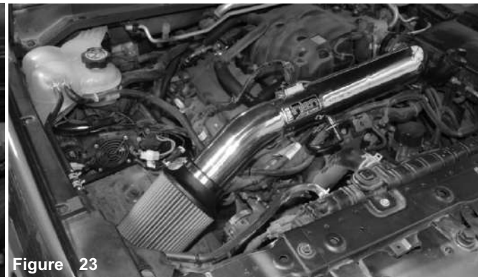
Figure 19 A) Install the intake tube into the vehicle and position the bracket to the vibramount and tube to the step hose.
