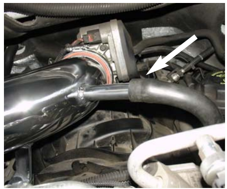
Connect the crank case line to the fitting on the intake tube and secure.
