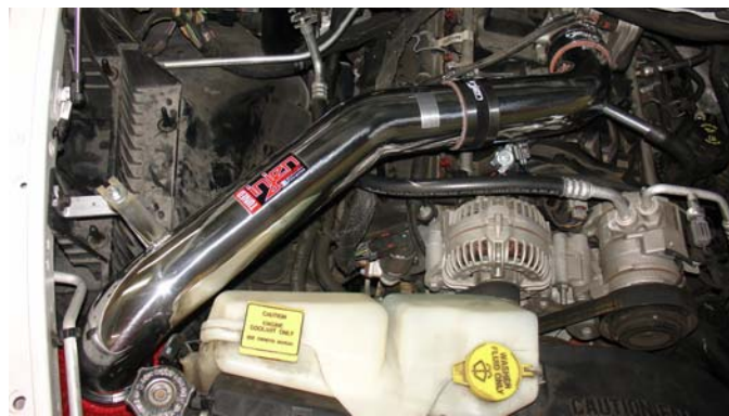
Check the entire air intake system for best possible fit, once proper clearance has been made through out the length of the intake, continue to tighten all nuts, bolts and clamps.
