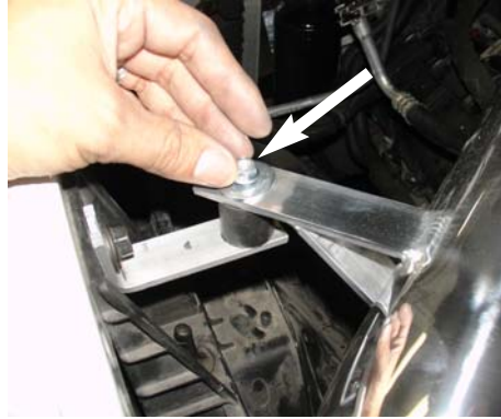
Secure the bracket to the vibra mount using M6 washer and nut.
