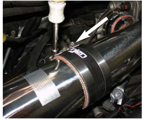
Position the intake for the best possible fit and clearance. Tighten all clamps using 8mm nut driver.
