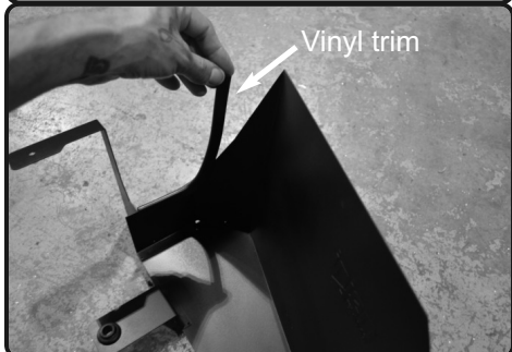
8. Install the provided Vinyl trim to the side of the heatshield.
