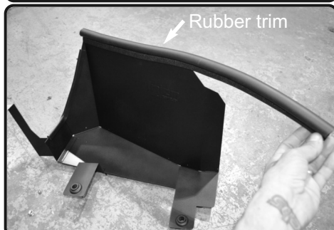
9. Install the Rubber trim to the top of the heatshield.
