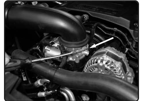
3. Loosen the clamp on the throttle body using 8mm nut driver.
