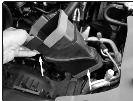
6. Carefully lift up and remove the front plastic scoop
