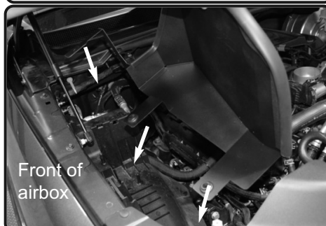
10. Install the heatshield assembly into the vehicle. position the tabs with grommets to the factory plastic studs.
