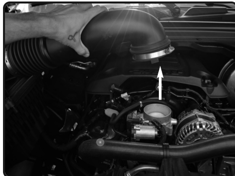
5. Pull back the intake tube from the throttle body.
