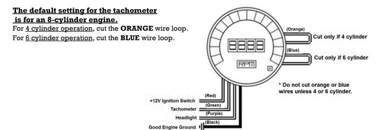
Ground - Black Connect directly to the engine block.
