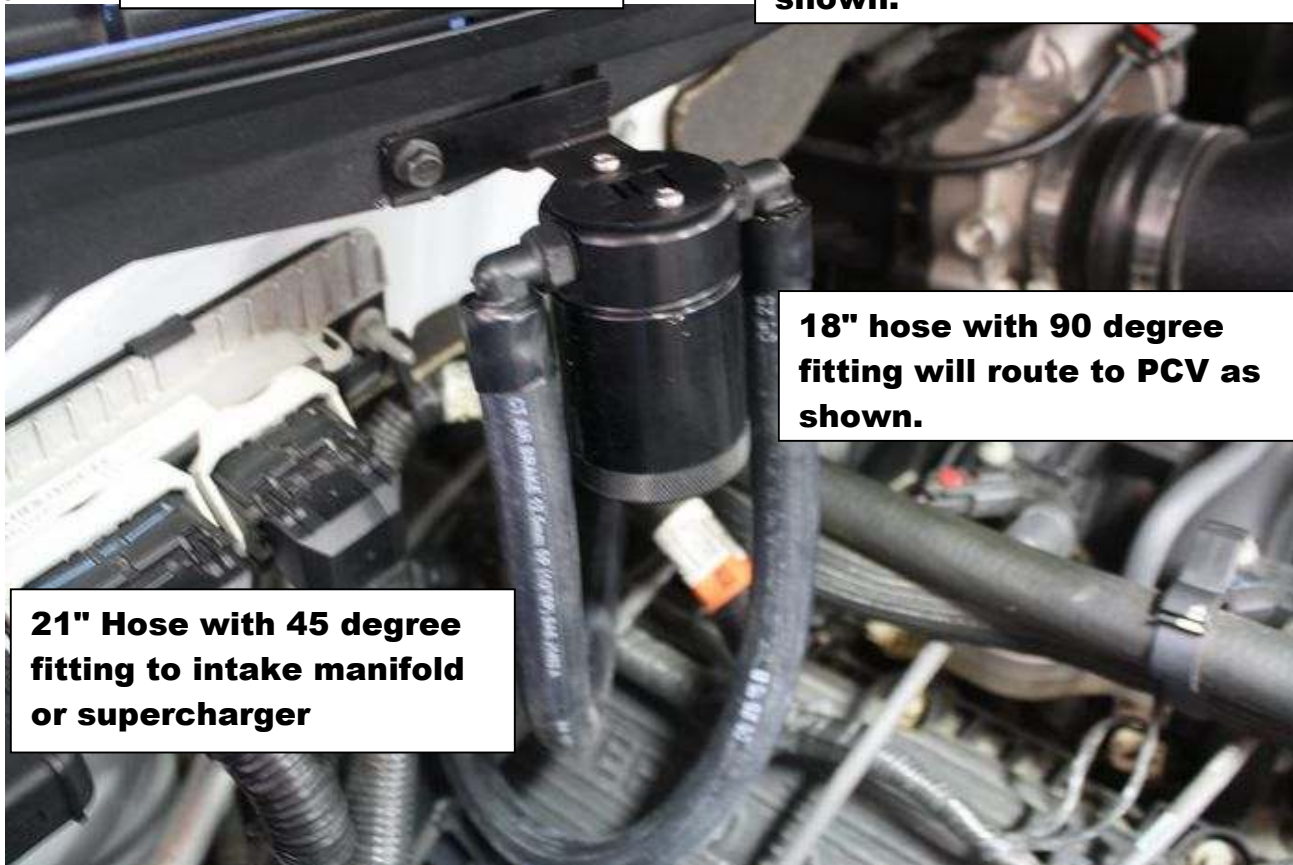
18" hose with 90 degree fitting will route to PCV as shown.
