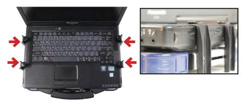
**4.1**) Locate the adjustment screw for each Side Clamp. Remove the lug by loosening the screw with the provided L-shaped Wrench.
