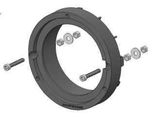
**6.** From the front of the bumper, Insert the new fog light and immediately align the chrome bezel over it. Align the three holes on the chrome bezel with the matching holes on the adapter bracket.
