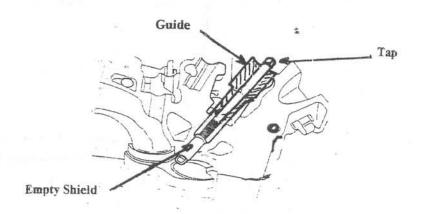
Once the ground electrode is tapped, insert the extractor through the guide and thread into the ground electrode shield. Place nylon washer and jam nut onto threaded shaft.
