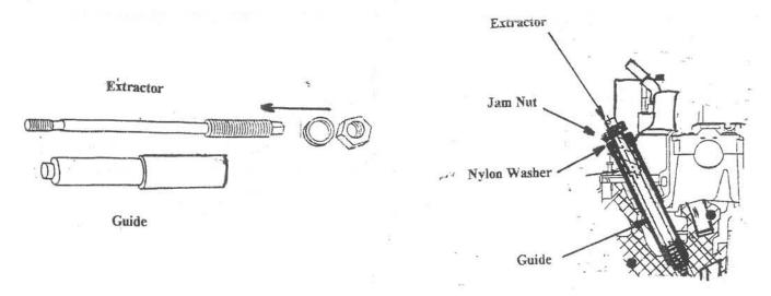
While holding hex end of extractor with wrench, turn jam nut with another wrench to remove ground electrode shield.
