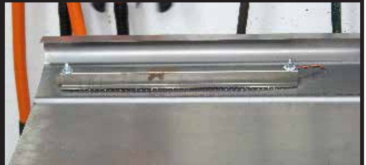
9. Attach the U-shaped bracket, with the LED bar, to the back of the panel and secure with lock washers and nuts.
