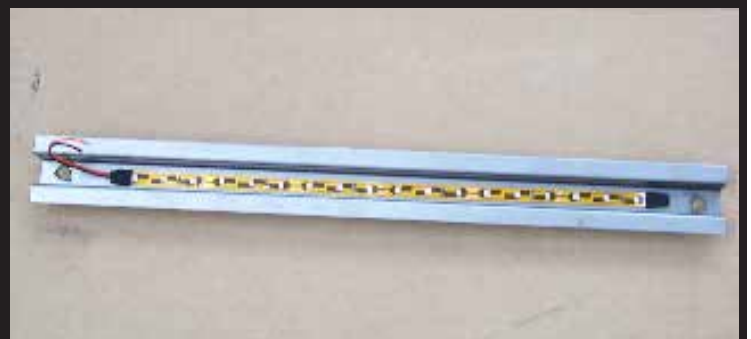
8. The Keep It Clean GhostLight LEDs line up and attach inside the U-bracket.
