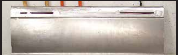
10. This is what the panel will look like once completed. The LED lights can be installed on any piece of sheet metal from a combo skin to a roll pan or tailgate.
