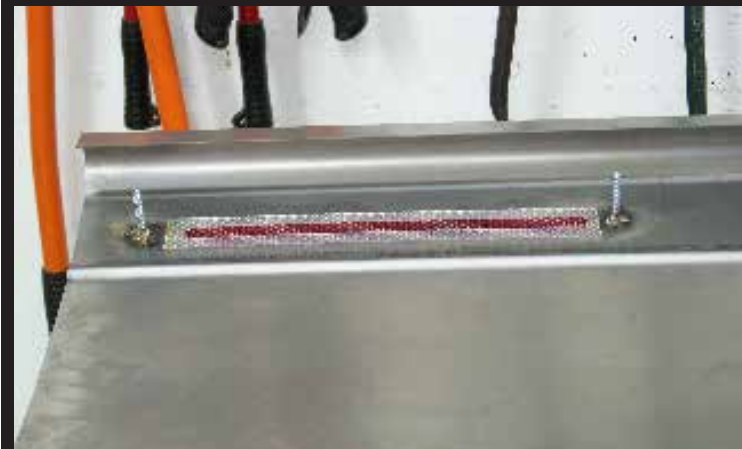
7. Attach the red Lexan insert to the clear diffuser and line up in the cut hole.
