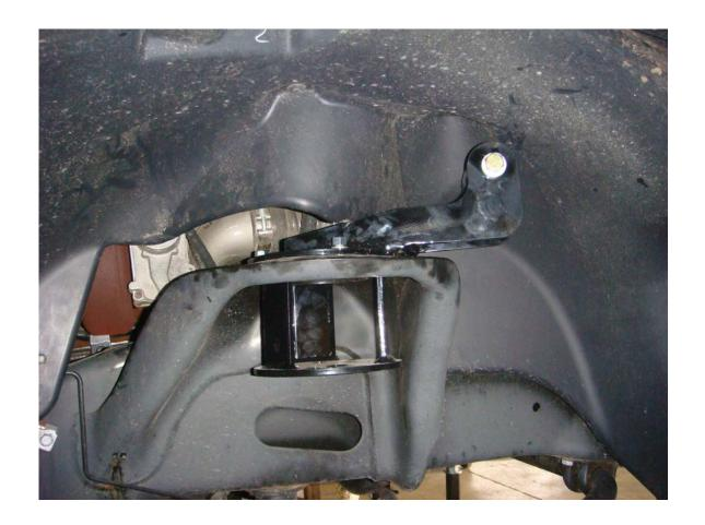
6. Locate the 5323 Firestone air bag. Next locate the lower air bag/lower shock mount. Fasten the air bag to the bottom mount with the 1/2x3 1/2" bolt and lock washer. Before torqueing the bolt, drop the assembly into place and jack up the axle to get the orientation of the top studs of the air bag with the top air bag mount. Once the bag location is determined, torque the 1/2x3 1/2" bolt to 35 ft/lbs.
