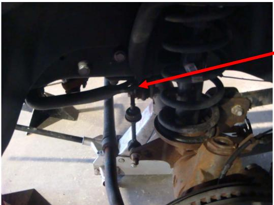
3. Remove the sway bar end link nut and pull off the rubber bushing.
