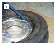
Stand on the tire and use the **curved end** of the tool to pry a section of the top bead over the rim
