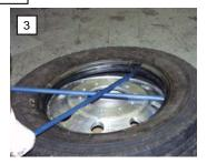
Once the two bars are crossed, forming an "X" over the rim, press down on the two bars. This will cause the first bead to demount.
