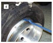
Lift the assembly as shown to partially release the wheel from the tire.
