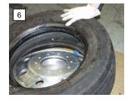
While holding **down** on the tire, lift the **curved end** of the bar to demount the second bead.
