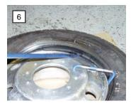
The **curved end** of the tool easily gets under the stretched bead for "that last bite".
