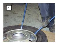
Break both beads and <u>always</u> use plenty of bead lubrication on the tire and wheel.
