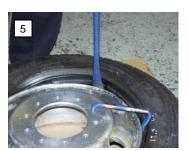
Repeat this step, taking small sections of the bead, until the last section is pried over the rim and the tire is mounted.
