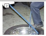
Start by bringing one **Nineteen-Five** bar across the center of the rim. Then cross with the second bar as you move to the opposite side of the tire/wheel assembly.
