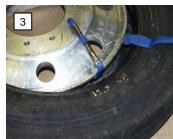
When mounting the top bead, place the bead holder (use #31710 for steel rims; #33196 (shown) for aluminum rims) on the rim and slide to one side, as a stop against the bead.
