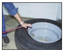
Keeping fingers out of the area **between** tool and tire/wheel, fully insert **small end**, between rim and tire bead nearest you, in top bead of tire.
