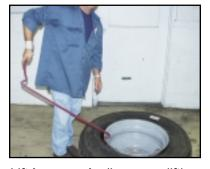
Lift large end. (Improper lifting will cause the tool to roll)
