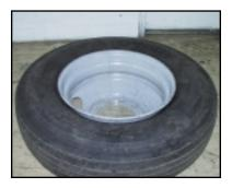
Break and lube both beads. Lay tire on floor with short side of wheel up.
