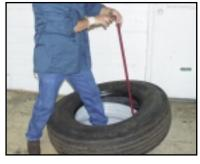
Lift **small end**, step through the wheel and pull tool across center of wheel.
