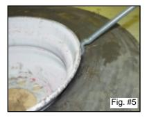
The small end of the tool easily gets under the stretched bead for that last pull.
