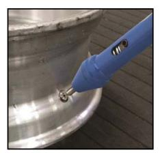
The Metric Valve Breaker allows wheel refinishing shops, truck tire service centers, as well as retreading shops, to have a specific tool to remove corroded and stubborn valve stems without spending time hunched over a wheel with a wrench and hammer.
