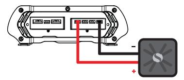
STEREO-AND-MONO-SIMULTANEOUSLY (SAMS) OPERATION minimum impedance of 4 ohms bridged (mono) and 2 ohms per channel stereo
