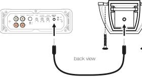
Remote cable passes audio; do not run cable parallel to power wires.
