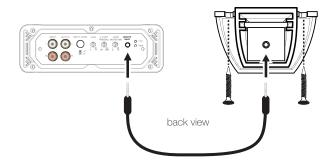
Remote cable passes audio; do not run cable parallel to power wires.
