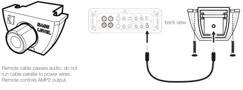
Connect the supplied 1/8th inch [3.5mm] patch cable to the CXARC remote and the Remote Bass jack on the amplifier
