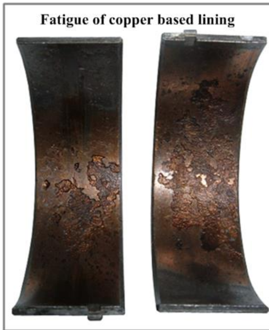
Fig.4 Fatigue of the copper based intermediate layer of tri-metal bearings
