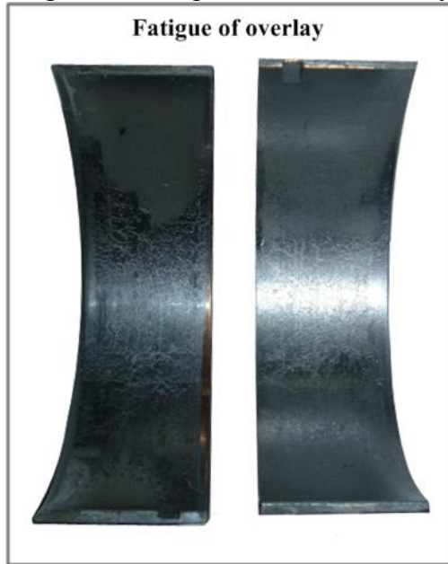
Fig.3 Fatigue of the overlay of tri-metal bearings
