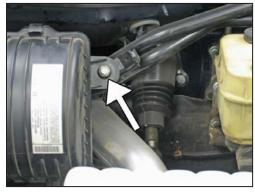
5. Remove the bolt that secures the filter housing to the support brace shown.
