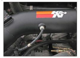
28. On vehicles equipped with a filter minder, connect the filter minder hose to the vacuum fitting installed in the K&N® intake tube in step #10.
