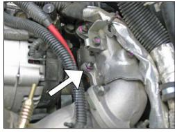
15. Remove the nut from the turbo intercooler inlet manifold mounting stud shown.
