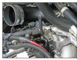
16.Install the secondary tube mounting bracket (26650) onto the intercooler manifold mounting stud and secure with the nut removed in step #15.
