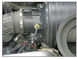
3. On vehicles equipped with a filter minder, disconnect the filter minder vacuum hose from the stock filter housing.
