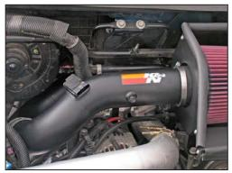
27. Install the secondary K&N® intake tube (27435) into the silicone hose at the primary tube, into the K&N® air filter and align with the tube mounting bracket installed in step #16. Secure the K&N® intake tube with the hose clamps and hardware provided.
