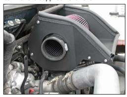
26. Install the heat shield side panel onto the main heat shield and secure with the provided hardware.
