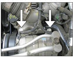
17. Remove the two A/C compressor pump mounting bolts mounting bolts shown.
