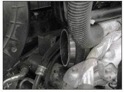
11. Install the provided silicone hose onto the turbo inlet tube and secure with the provided hose clamp.
