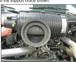
6. Remove the filter housing from the vehicle.
