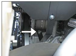
23. Secure the heat shield side bracket to the forward threaded hole next to the A/C compressor as shown with the provided hardware.
