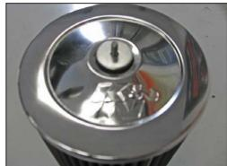
24. Install the supplied rubber washer and fender washer onto the stud protruding from the filter lid as shown.
