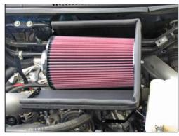
25. Install the K&N® air filter into the heat shield so the mounting stud protrudes through the heat shield and the mounting bracket. Then secure the filter with the supplied hardware.
