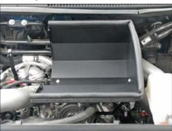
22. Install the heat shield onto the mounting bracket on the A/C compressor and secure with the provided hardware.
