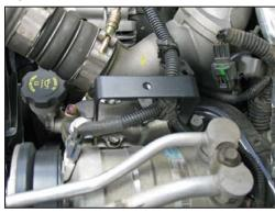
18. Install the heat shield mounting bracket (26644) onto the A/C compressor and secure with the bolts removed in step #17.
