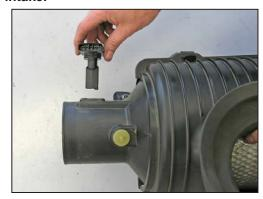
8. Remove the two screws that secure the mass air sensor to the stock filter housing and then remove the mass air sensor as shown.
