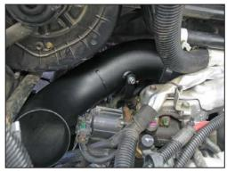
13. Install the primary K&N® intake tube (27434) into the silicone hose at the throttle body and align with the mounting bracket installed in step #12. Secure the primary intake tube with the hose clamp and hardware provided.
