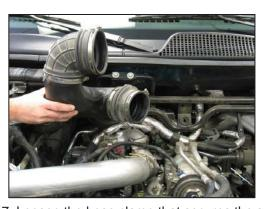
7. Loosen the hose clamp that secures the stock intake tube to the turbo inlet tube. Then remove the complete intake tube assembly from the vehicle as shown.
