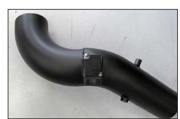
9. Install the mass air sensor into the secondary K&N® intake tube and secure with the provided hardware.
