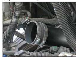
14. Install the silicone hose (08698) onto the primary intake tube and secure with the provided hose clamp.
