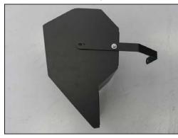
19. Install the heat shield mounting bracket onto the heat shield and secure with the provided hardware as shown.
