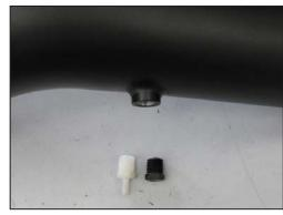
10. On vehicles equipped with a filter minder, install the ¼"npt vacuum fitting into the K&N® intake tube. On vehicles without a filter minder, install the ¼"npt plug into the K&N® intake tube.
