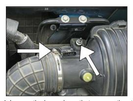
4. Loosen the hose clamp that secures the stock intake tube to the filter housing and then remove the nut that secures the filter housing to the support bracket.
