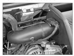
26. Reconnect the mass air sensor electrical connection.
