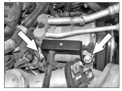
15. Install the heat shield mounting bracket (26644) onto the A/C compressor and secure with the factory bolts removed in step #14.
