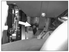
20. Secure the heat shield side bracket to the forward threaded hole next to the A/C compressor as shown with the provided hardware.
