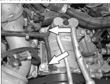
14. Remove the two A/C compressor pump mounting bolts shown.
