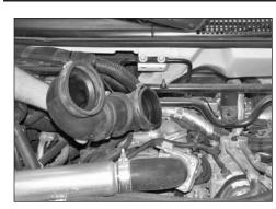
7. Loosen the hose clamp that secures the intake tube assembly to the turbo inlet tube. Then remove the complete inlet tube assembly from the vehicle as shown.
