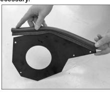
18. Install the small edge trim onto the heat shield wall as shown.
