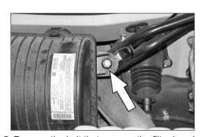
5. Remove the bolt that secures the filter housing to the support brace shown.
