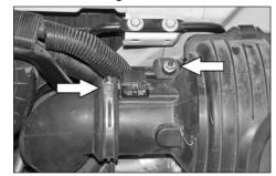
4. Loosen the hose clamp that secures the stock intake tube to the filter housing and then remove the nut that secures the filter housing to the support bracket.
