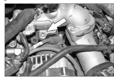
12. Remove the nut from the intercooler manifold mounting stud shown.
