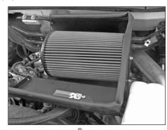
22. Install the  $K\&N^{\otimes}$  air filter into the heat shield so the mounting stud protrudes through the heat shield and the mounting bracket. Then secure the filter with the supplied hardware.
