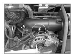
25. On vehicles equipped with a filter minder, connect the vacuum line to the  $\frac{1}{4}$  npt fitting installed in the K&N  $^{\circ}$  intake tube as shown.
