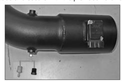
10. On vehicles equipped with a filter minder, install the 1/4" npt vacuum fitting into the K&N<sup>®</sup> intake tube. On vehicles not equipped with a filter minder, install the 1/4"npt plug into the K&N<sup>®</sup> intake tube.
