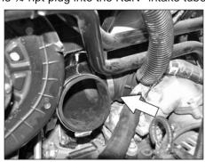
11. Install the 90° silicone hose (084088) onto the turbo inlet and secure with the provided hose clamp. NOTE: The K&N® logo should be installed towards the turbo inlet. Do not completely tighten at this time.
