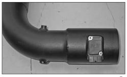
9. Install the mass air senor into the K&N<sup>®</sup> intake tube and secure with the provided hardware.
