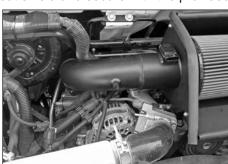
24. Install the K&N<sup>®</sup> intake tube into the silicone hose and into the K&N<sup>®</sup> air filter, align the tube with the mounting bracket installed in step #13. Secure the intake tube to the filter and silicone hose with the provided hose clamps and to the mounting bracket with the provided hardware.
