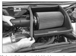
23. Install the heat shield side panel onto the main heat shield and secure with the provided hardware.
