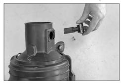
8. Remove the two screws that secure the mass air sensor to the stock filter housing and then remove the mass air sensor assembly.
