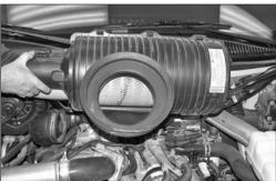
6. Remove the filter housing assembly from the vehicle.
