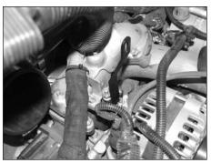
13. Install the tube mounting bracket (26650) onto the intercooler mounting stud and secure with the nut removed in step #12.
