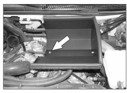
19. Install the heat shield onto the mounting bracket on the A/C compressor and secure with the supplied hardware.
