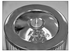
21. Install the supplied rubber washer and fender washer onto the stud protruding from the filter lid as shown.
