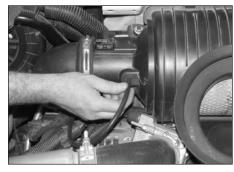
3. On vehicles equipped with a filter minder, disconnect the filter minder vacuum hose from the stock filter housing.
