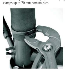
The spring hose clamp pliers reliably grip standard, space-saving and wire clamps as well as spring band
