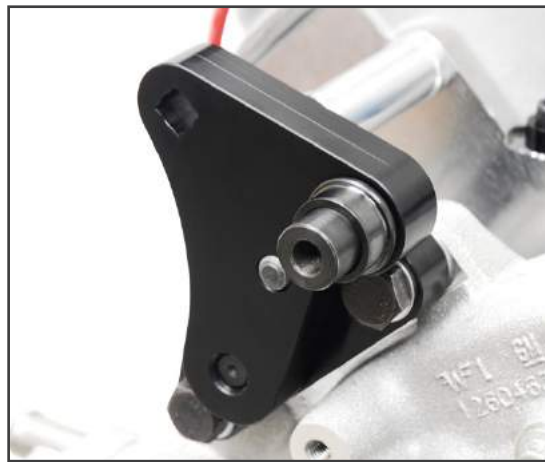
The Idler pulley spins on a steel shaft providing extra strength & support for the pulley.
