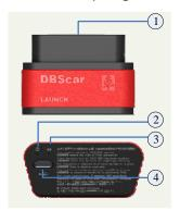
Fig. 1-3 DBScar diagnostic connector
