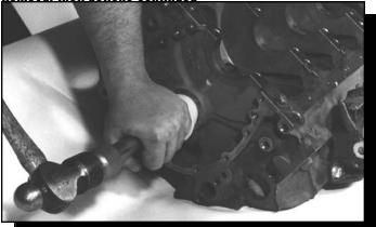
**Step 5** - Place nylon cone in first bearing housing and drive bearing out. Loosen driver assembly to relieve pressure and pull tool back through the next bearing to
