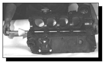
**Step 4** - Operate tool from front of block. Insert into rear bearing and tighten until snug in bearing. (over)
