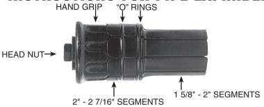
Holding tool by handgrip, insert it into pipe. If pipe is less than 2" diameter, the small end is used. On pipes 2" and over, push right on in until the large segments will contact. Expand by turning head nut with a wrench. Tool will expand smoothly and easily and will round up pipe end quickly. The tool does not turn in the pipe.
