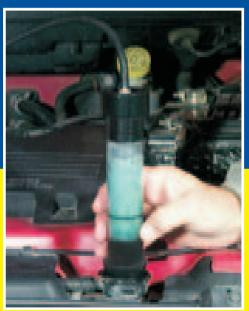
Tester Operates on Engine Vacuum with Silver Breather or with a Hand Vacuum Pump using Red Breather
