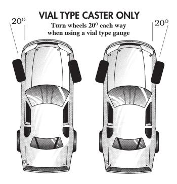
NOTE: Adjusting the caster may have an effect on the camber and vice versa. Double check all your settings before finishing. Be sure to tighten all suspension bolts when done.
