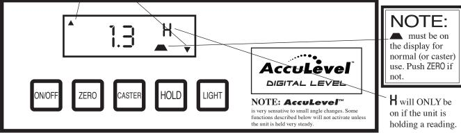
**NOTE:** This Ver. 5 **Acculeve** I<sup>™</sup> has 2 modes of operation. 1) In Normal angle measurement mode the display is steady. 2) In Caster Mode the display flashes (and will not measure absolute angles). Push CASTER button to exit Caster mode and go back to Normal angle measurement.
